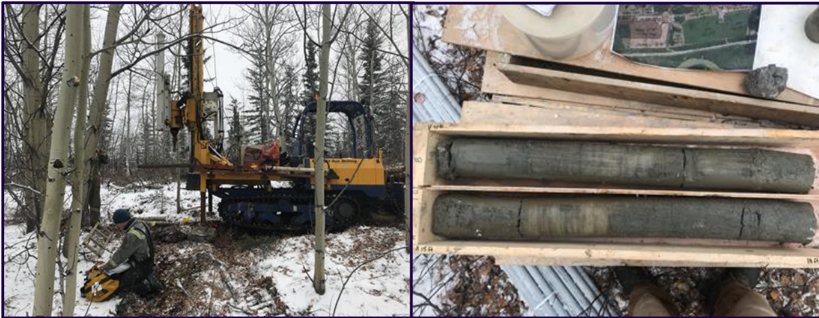
Figure 6. Midnight Sun Drilling CRREL drill rig and permafrost cores (WH_1456_BH1)
