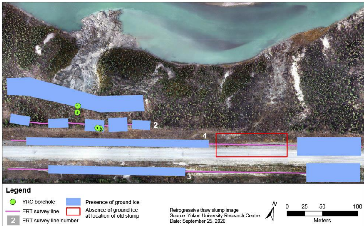
Figure 37. Approximate position of ground ice based on ERT profiles
