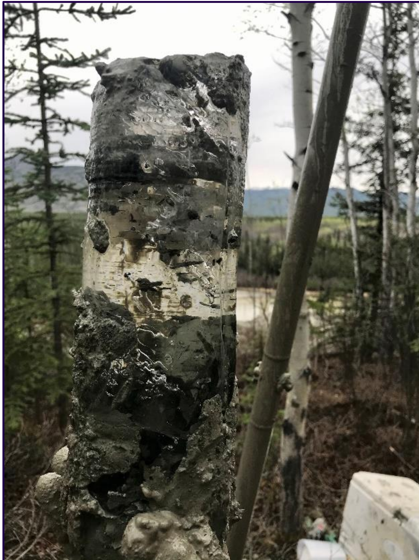
Figure 16. Ice rich permafrost core showing suspended cryostructure collected from borehole WH_1456_BH03
