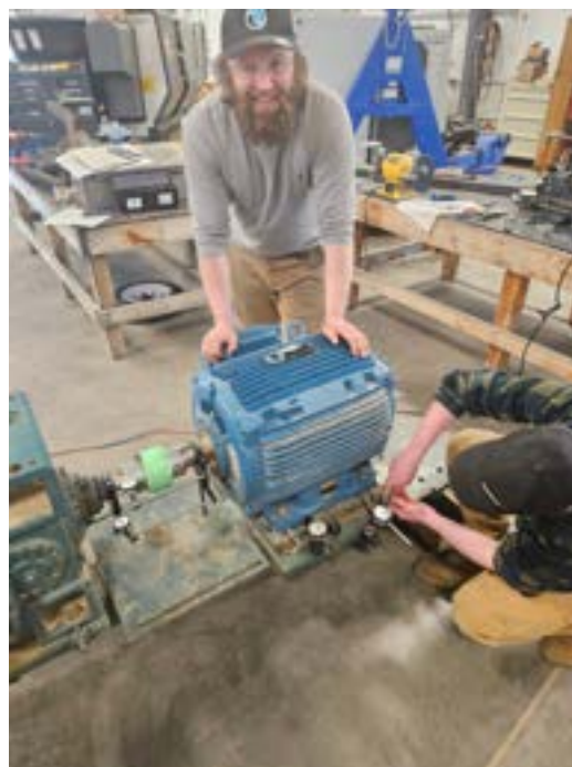
Pre-Apprenticeship Millwright students Pelly Vincent-Braun and Axel Buchanan conducting a motor alignment.
