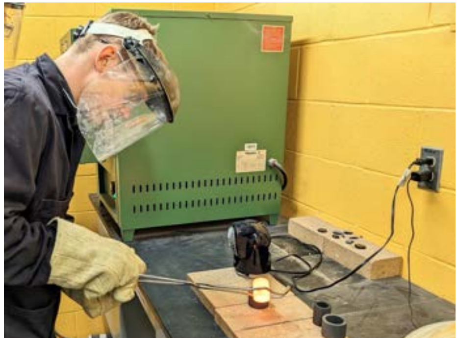
Earth Sciences student, Kieran McClenahan, conducting whole-rock fusion on Minto mine ores under the guidance of Dr. Cubley.
