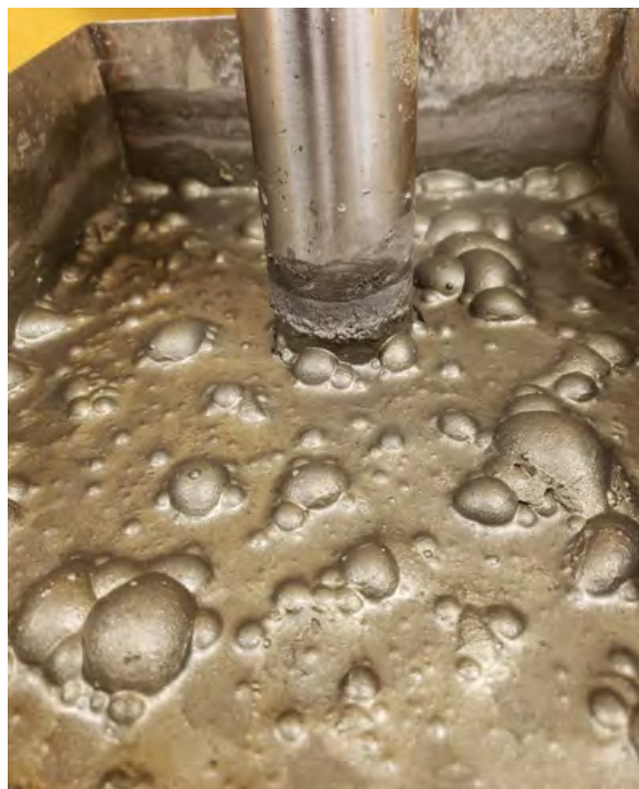
Laboratory-scale froth floatation tank separating copper sulphide minerals in the Earth Sciences Laboratory.
